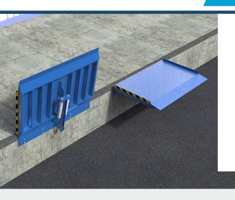
Folding bridges are designed for unloading of railway cars or for unloading trucks when there is no possibility to park close to the ramp. Folding bridges are installed on an open ramp in a stationary or sliding design, compensating for the difference between the ramp and the body of the cargo platform. The lifting capacity of the STL folding bridges is up to 4 tons.
