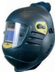
Helmet shell made of heat/cold resistant SUPER Termotrek® material equipped with fabric seal reliable protects welder's face and neck against sparks, metal spray and arc radiation. Automatic welding filter (110x90x5 mm) protected outside by panoramic PC cover lens and non-fogging back plate inside. Mass: 500g.
