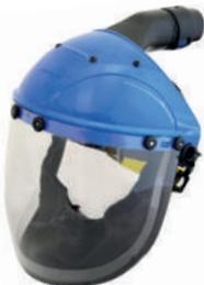
Enlarged visor with fabric seal is made of 2mm thick PC or CA (1.6 mm thick). Both visor options has anti-fog and hard coating, forehead made of heat/impact resistant material. Visor optical class one, mass: 350g.
