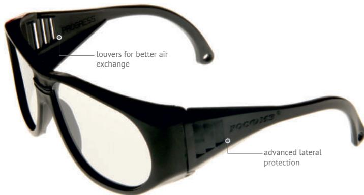
Universal protective spectacles providing protection against hard particles impact (0.5 J, V=5.1 m/s). Reliable plastic frame, widened temples with louvers for ventilation, temple length adjustment, lateral protection due widened temples, hardened mineral lenses.
