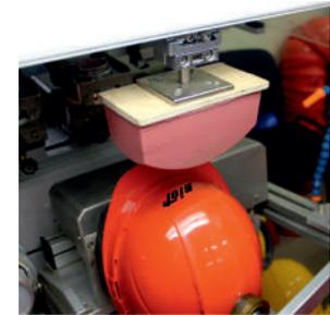
**Pad printing** is a modern technology of logo application based on paint transfer to the subject by means of elastic silicone pad capable to coincide with subject surface curvature. The modern pad printed equipment is launched and run at our plant.
