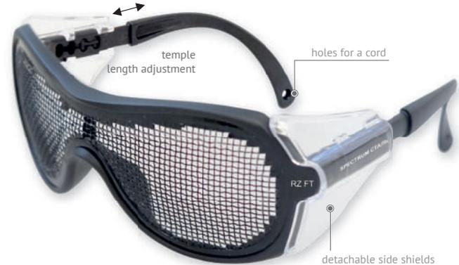
Protective spectacle with ocular made of steel wire mesh (cell size 2 x 2 mm) painted with black enamel for rust prevention. Provides protection against high speed particles (low energy impact  $V=45$  m/s).
