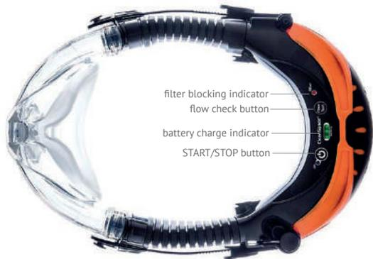
This PAPR protects against aerosols, gases and their combinations, its intelligent breathe responsive flow control system allows to spare battery charge: air flow is increasing at intensive breathing and decreasing at quiet breathing
