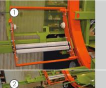
A carriage is equipped with a tensioning unit for tight wrapping of bales.
