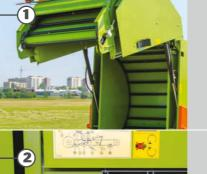
Constant volume chamber forms the high-density bales having an ideal cylinder shape. It has an increased number of pressing shafts made of high alloy steel: shafts and chains provide pressing of high humidity grass chopping.
