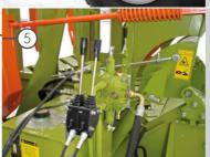
An independent hydraulic system excludes use of an offgrade lube from a tractor hydraulic system. A remote control system allows controlling the bale cutter from a tractor cab.
