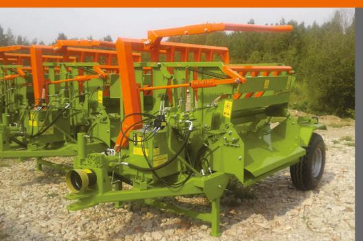
The initial option of the bale cutter supplied from Italy was a 4 wheeled one (IRK-01). In 2003, with due account to a condition of roads at farms in Russia and more than 8 years of experience in equipment exploitation at Russian farms, a new modification of the bale cutter on two wheels of larger diameter was master manufactured (IRK-01.1).
