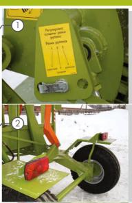
The cut length can be adjusted within the range of: 9-15-22 cm.
