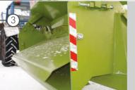
An extra dismountable chute allows using the bale cutter in farms where high trough feeders are installed.
