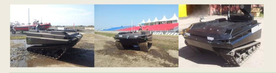
Multifunctional robotic platform "Pellets-MRP" with automatic remote control can be installed on any of the ATV "Pelec". Movement control modes:
