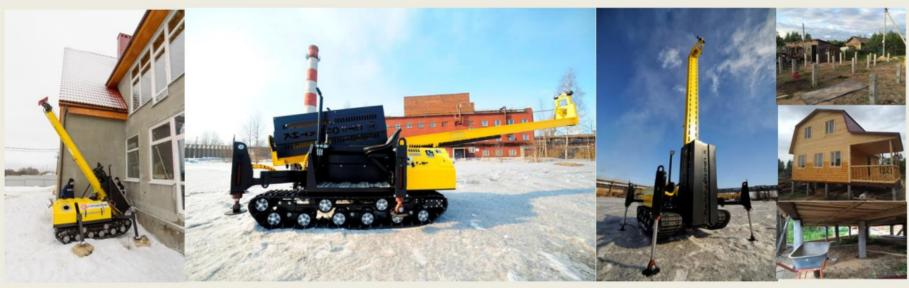
Pile-driving plant develop a new market segment - the construction of foundations on reinforced concrete piles for low-height housing construction. This is the first model of a compact size pile-driving machine on the caterpillar track, which is suitable for working in residential areas and preserves the customer areas from damage. The compact dimensions of the unit allow to move it in car trailer.
