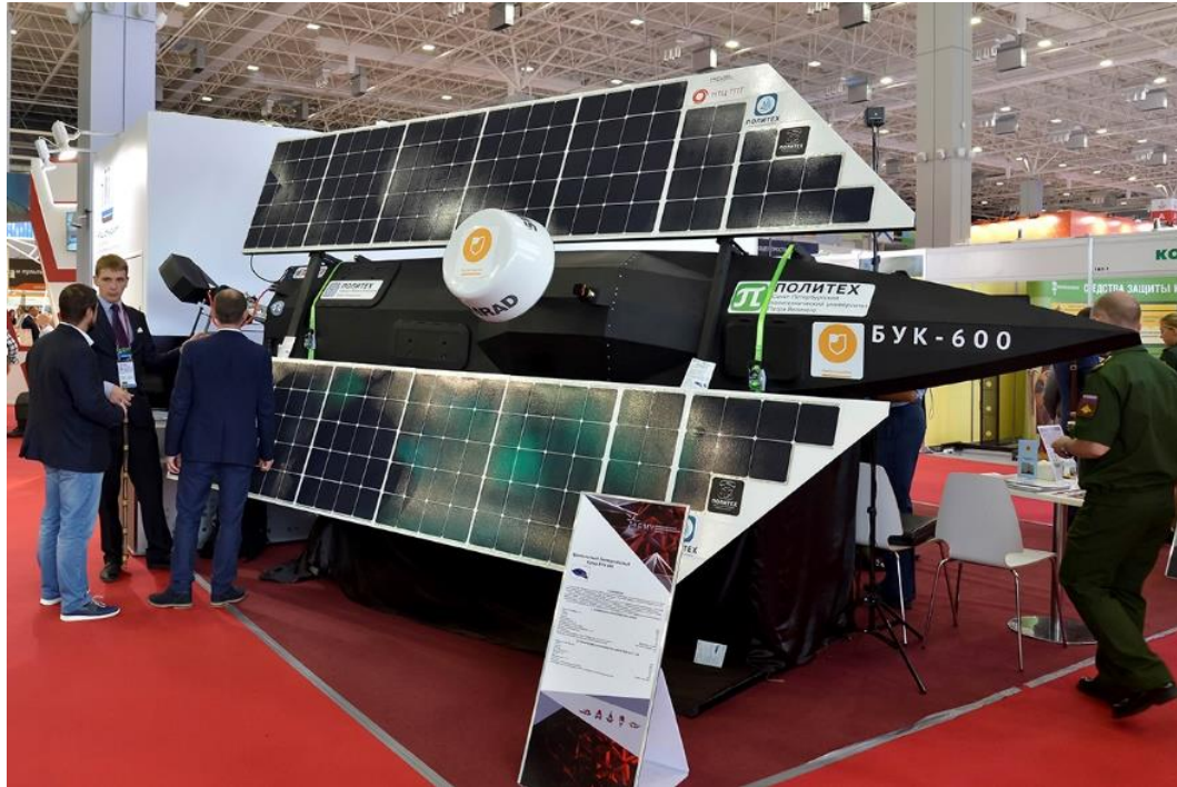
Multipurpose self-driving powerboat developed at Peter the Great St. Petersburg Polytechnic University
