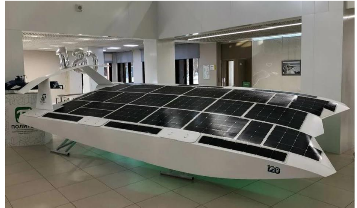
Hydrofoil self-driving solar boat "Storm-600" developed at Peter the Great St. Petersburg Polytechnic University
