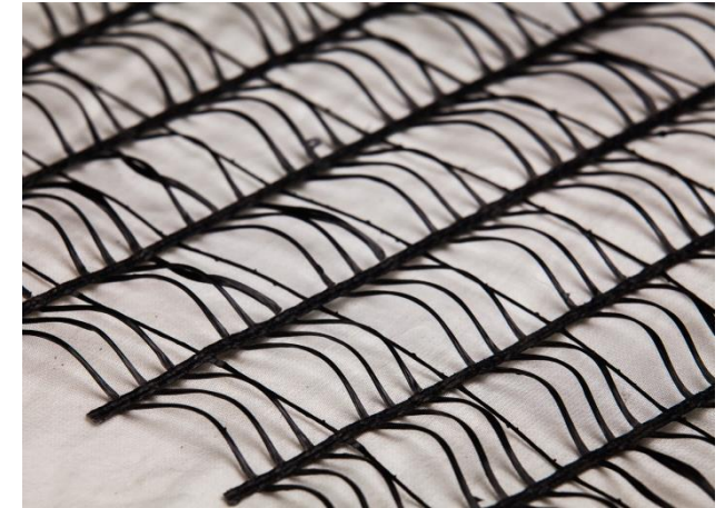
Polypropylene geomat with a glass/polyester impregnated geogrid backing, strength up to 100 kN/m
