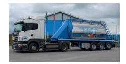
and "Sibirit-1200", of emulsion and gas generating agent, as well as water spray solution with subsequent reloading of these components into mixing-charging trucks. Tank semi-trailer's loading capacity is 27 tons of components.
