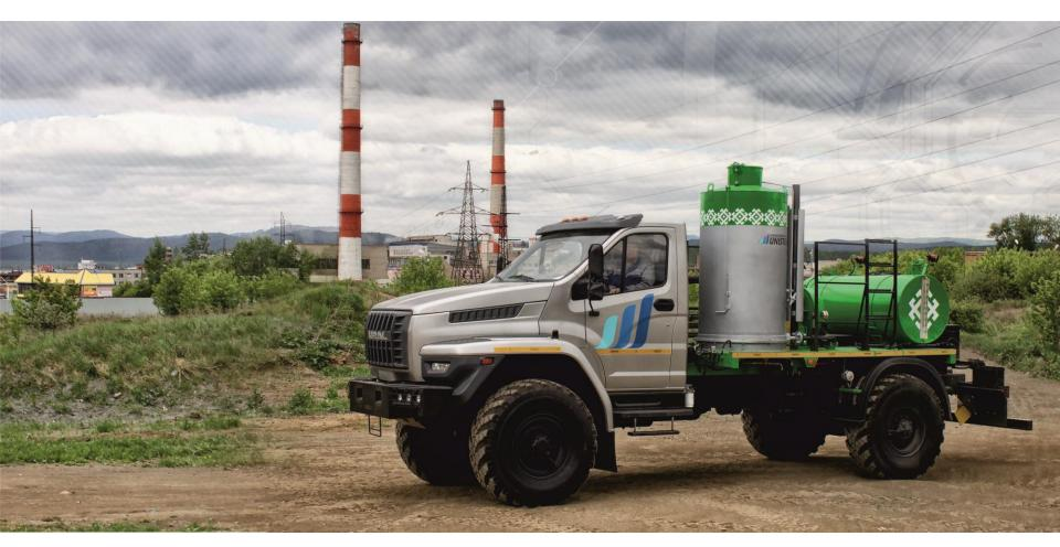
Thermal bed stimulation prevents the formation of wax and gum deposits in pore space of oil stratum and facilitates the volume of current and total oil extraction. Thermal treatment of well-bottom zone extends the useful life of oil well, as the increase in oil temp. reduces its viscosity and wax deposits inside producing pipelines. Oil-well Dewaxing Unit effectively tackle the task of increase and recovery of productivity of oil-well, and dewaxing of equipment and pipelines.
