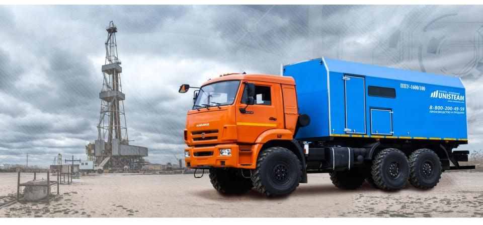
Mobile Steam Generator is adjusted to the truck chassis. Steam generator is arranged on the adjusted platform and is protected from the dust and weather conditions by the steel box carrier. The operational mode is remote and is performed whether from the driver's cabin, operator's room or inside box carrier. The steam generator is powered by the automobile engine or electric engine. Steam boiler, burning device, high-pressure fan, water pump and fuel pump are arranged on the adjusted platform.
