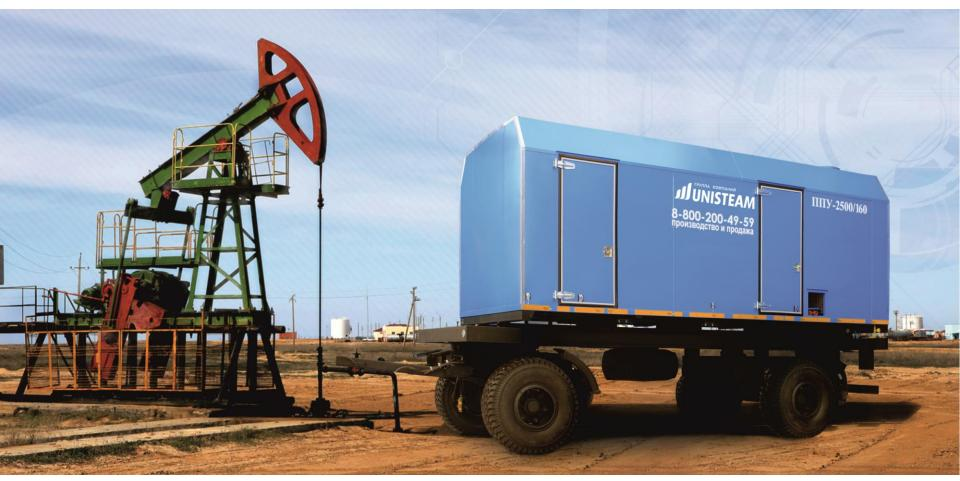
Trailer-Mounted Mobile Steam Generator is a compact version of truck-mounted model. Allows fully autonomous operation being powered by diesel generator. To enable maximum comfort an operator's room can be provided. Perfectly deals with thermal treatment of oil well by steam loads, as well as industrial cleaning of equipment by streamlining steam via spray head.
