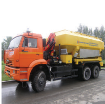
MSZ-15-NP-K with a side-mounted sweep auger
