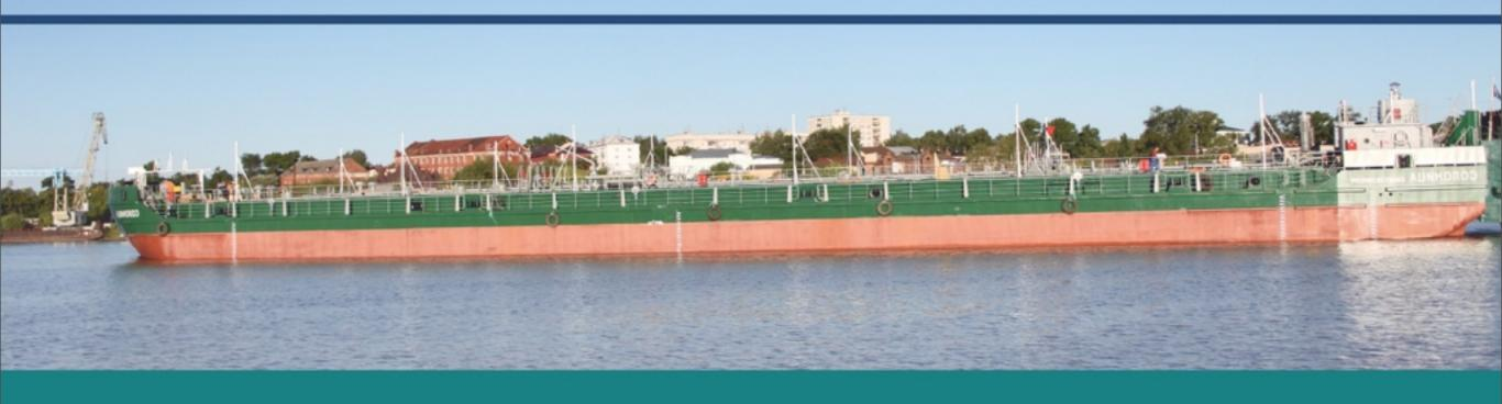
The vessel is designed for transportation of petroleum products with vapours flash points of below and above 60' C, including products that require heating. RMRS class notation:KE R3-RSN Oil tanker.
