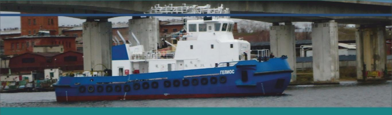
Designed for towing and pushing barges with cargo capacity of 5000-8000 t carrying all kinds of oil, including crude oil and oil products with vapour flash point below 60' C. Class RMRS KM R2-RSN Ice2 AUT3 Tug.
