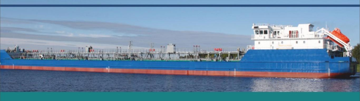
The vessel is designed for transportation of petroleum products without vapours flash point restriction, including those requiring heating.
