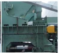
Concrete plates or any other construction wastes are pushed on the table to be pressed. Once concrete slab crushed, the rebar is moved to the output. The stones crushed go through the output trays toward the conveyer and are shipped for further processing.
