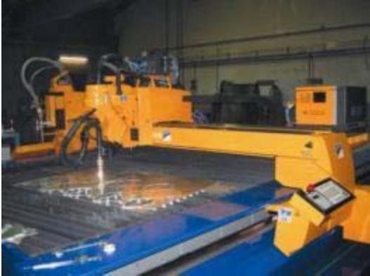
Cutting machine with plasma and oxygen. The working surface of 2500 x 21000mm
