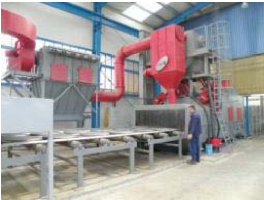
shot-blast cleaning plant - width 2500, height 650
