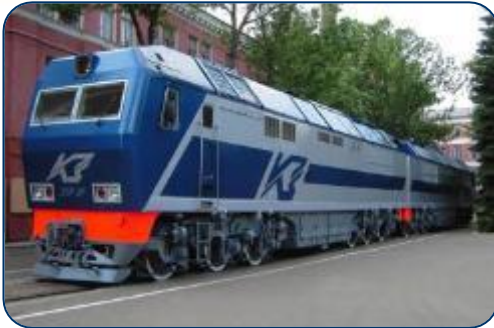
2TE70 with collector traction motors
