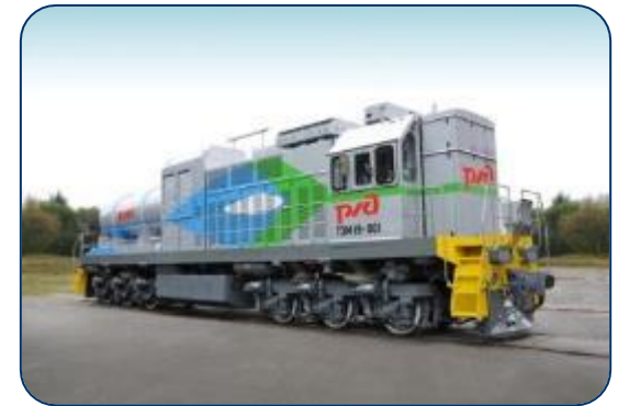
TEM19 with gas reciprocating engine
