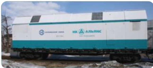
EGN1000 power plant
