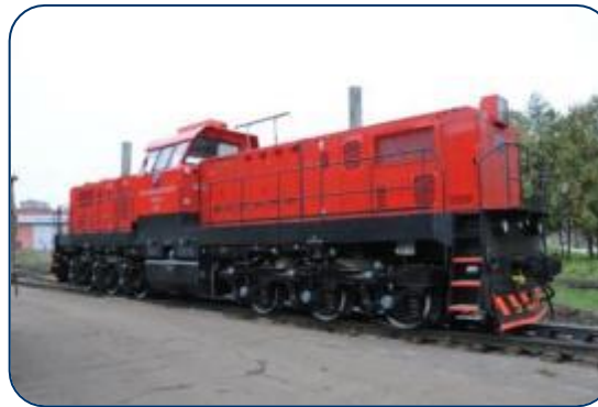
TEM33 with dual diesel power unit
