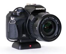
sticker and of sensor, which is fixed on the good by means of a screw and is twisted into the photocamera tripod hole.
