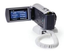
Sensor is inserted into support and allows to take a good into the hands freelv. Support and sensor connected by twisted cable. A screw, twisted into a tripod hole, closes the circuit, and the protection system will produce sound sygnal if any unauthorized attempt to remove a good from the sensor occurs.
